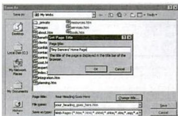
Saving your first Web page, with a file name and a title.
